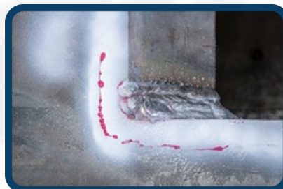
Penetrant Testing (PT):
