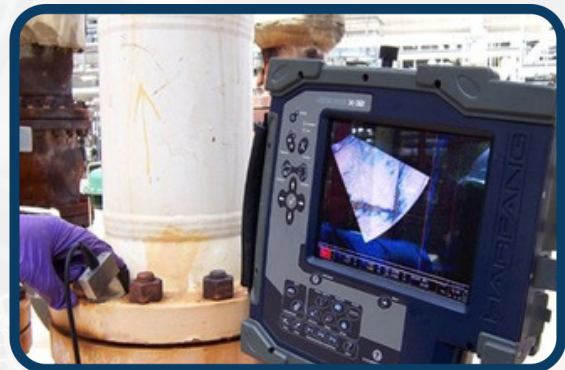
Phased Array Ultrasonic Testing (PAUT):
